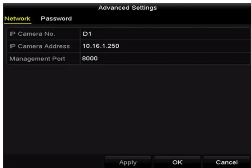
Figure 2-33 Network Configuration of the Camera
