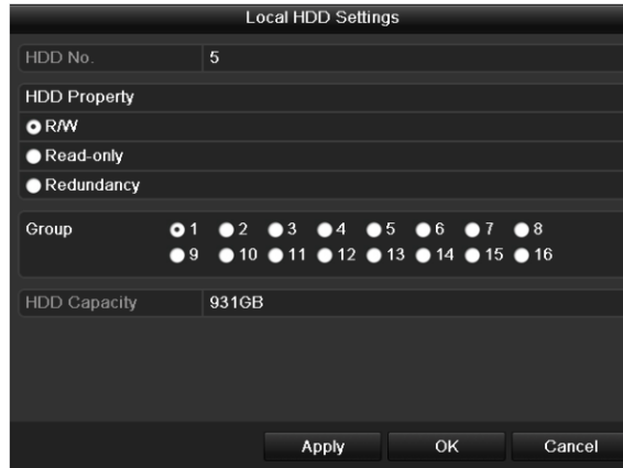
Figure 12-13 Local HDD Settings Interface
