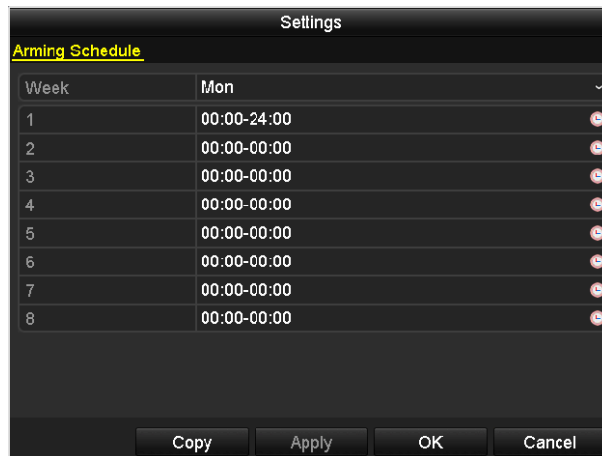
Figure 8-17 Set Arming Schedule of Alarm Output
